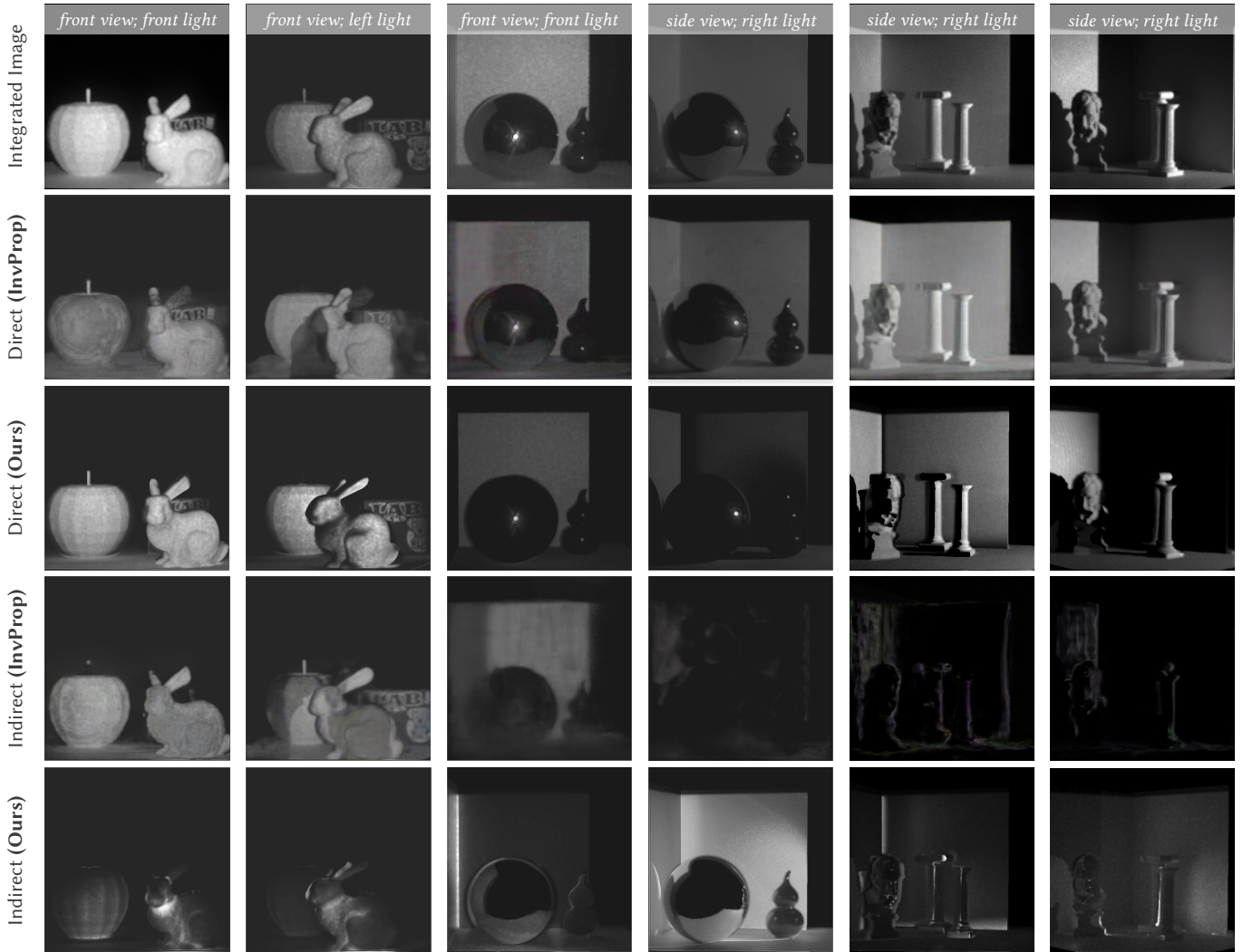
Fig. 12. Separation of direct and indirect light transport under different illuminations, and from different viewpoints. While InvProp relies on volumetric rendering and implicit neural caches, our framework leverages explicit geometry and the Transient Rendering Equation to rigorously disentangle light paths. By enforcing physical consistency, we achieve a sharp separation, particularly between direct metallic specular reflections and indirect scattering effects on the back walls.
